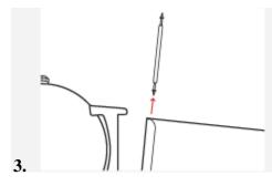
Take out the springbar and place the springbar on the side. Follow the same step to remove the strap on the opposite side of the watch.
