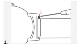
Press down on the spring bar tool and pull it slightly inwards towards the center of the strap. This will eventually loosen and detach the spring bar from the strap.
