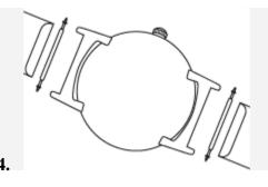
After you have taken out all the straps, take the new straps and place it in between the notches to insert the spring bar.
